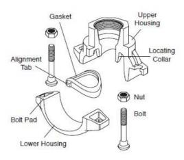
When bolts are tightened with a proper torque, the outlet housing makes metal to metal contact with the outer surface of the pipe.
